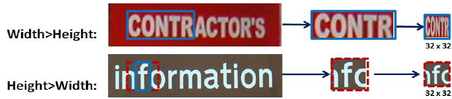
Figure 5.3.2: Patch extraction from detected MSER components. Patches of size 32-by-32 are extracted and given to the classifier to generate the detector scores. Image based on [HQT14].
