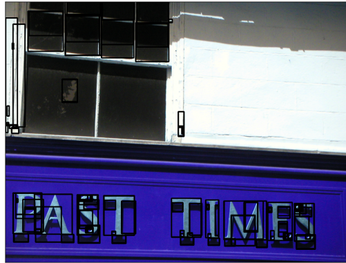
Figure 6.1.1: Detected maximally stable extremal regions in an image. Each detected region is surrounded by a rectangular bounding box. The height and width of the MSER are determined from the height and width of the rectangular bounding box respectively.
