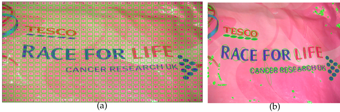
Figure 3.3.1: Dense Sampling Vs MSER Detector. Figure (a) shows the interest points detected by dense sampling. Here the stride is selected to be greater than the receptive field for better visualization. The detected keypoints are denoted by black dot. Figure (b) shows the keypoints detected by MSER detector from same image. MSER regions detected are denoted by green ellipses. and the keypoints are represented by green 'plus' symbol. It is evident that in case of interest point operators large part of the image is unsampled.
