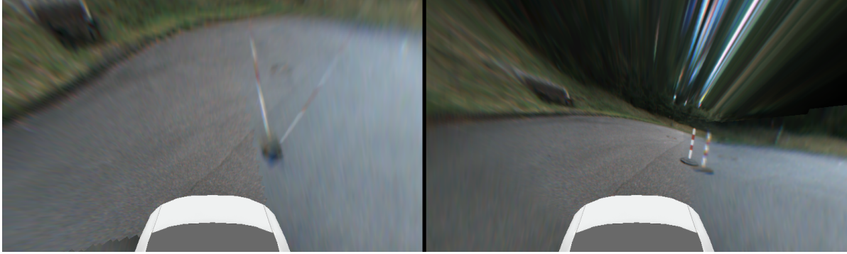
Figure 4.6.9: Free as handle Deformation including ground plane (obstacle in Back-Right Region) - Image provided by Robert Bosch Car Multimedia GmbH
