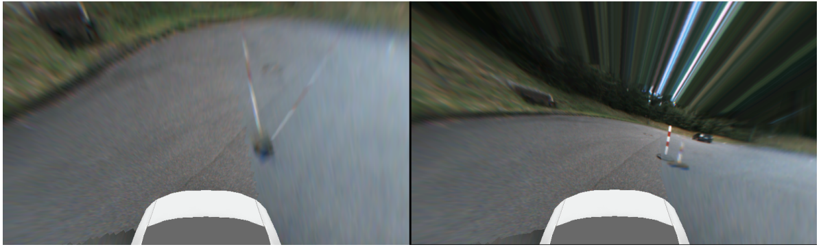
Figure 4.6.5: Constrained Deformation including ground plane (obstacle in Back-Right Region) - Image provided by Robert Bosch Car Multimedia GmbH
