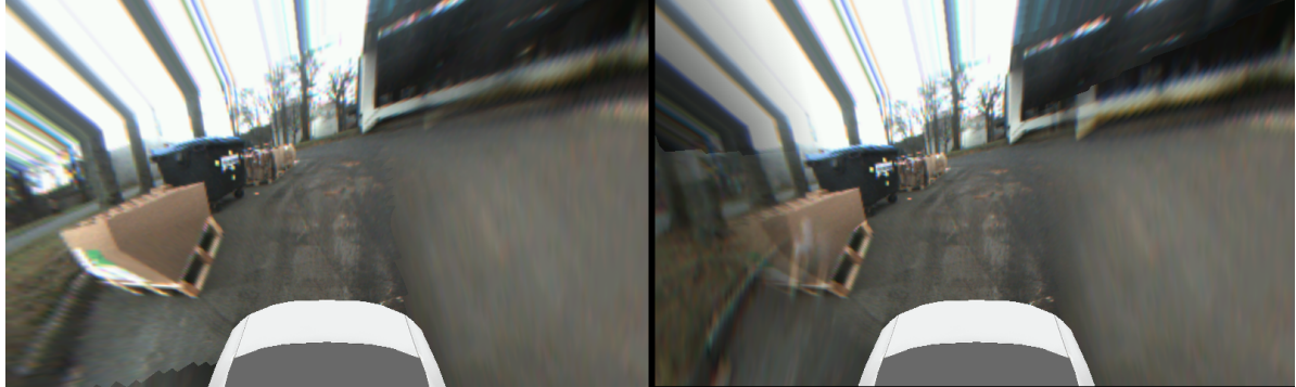
Figure 4.9.3: Effect of Number of Correspondences on Visualization - Left Image is a Frame with all 6 Correspondences, Right Image is the same Frame with only 1 correspondence at random having lowest SSIM Index of 0.64 for the Crate Obstacle - Image provided by Robert Bosch Car Multimedia GmbH
