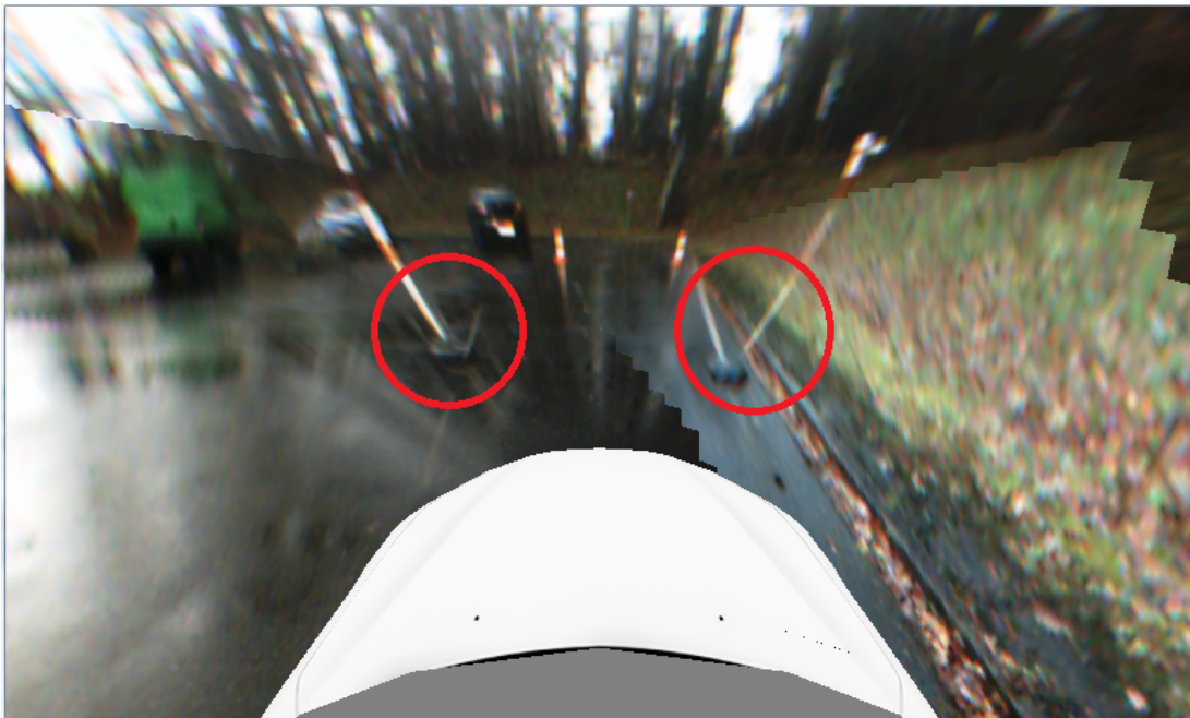
Figure 1.1.2: Visualization on Head Unit of the parking scenario with imaging artefacts introduced (two poles are seen instead of a single pole at both locations) - Image provided by Robert Bosch Car Multimedia GmbH
