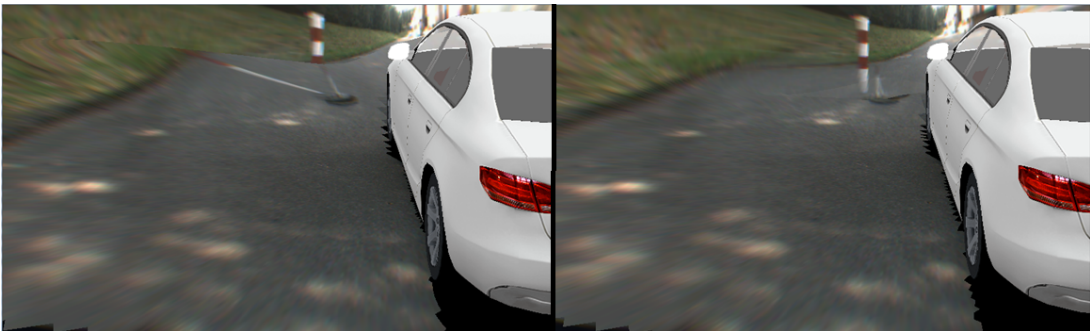
Figure 4.6.2: Deformation using ground plane (The left image is the undeformed View and the right image is the deformed view) - Left View - Image provided by Robert Bosch Car Multimedia GmbH
