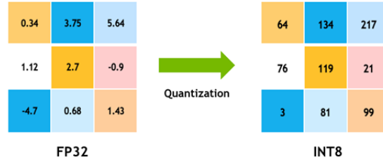
Figure 3.1.1: Example of FP 32 accuracy achievement for INT8 inference Using Quantization. Figure taken from [NZ21].
