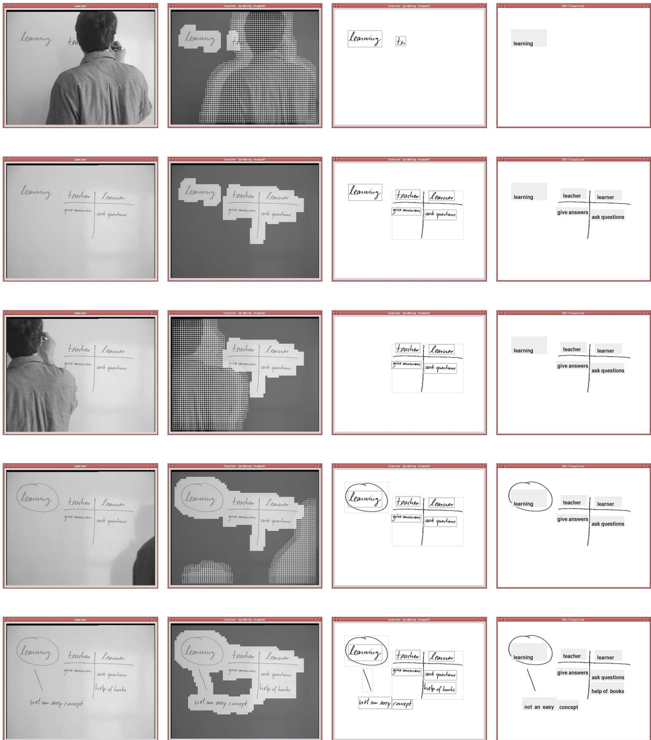
**Fig. 2.** Snapshots of an example image sequence. First column: grabbed images. Second column: distinction of text, background and noise regions based on the block partition of the image. Third column: clustering of binarized text components to words or phrases, respectively. Fourth column: results of text recognition.
