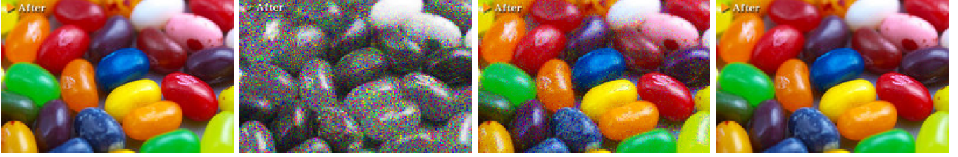
Figure 2. Example of the influence of the randomization parameters p_b and p_s . Left-to-right: original image, image randomized with p_s = p_b = 0 , p_s = p_b = 1 , and p_s = p_b = 4 . As can be seen, increasing the parameters p_b and p_s improves the perceptual quality up to the point that no visual difference can be perceived.
