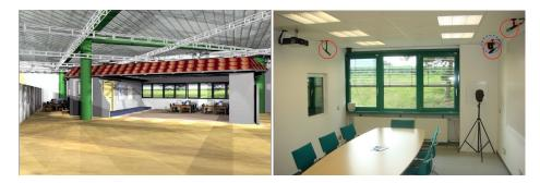
**Fig. 1.** Overview of the FINCA (left) and inside view of the smart conference room. Ceiling mounted microphones are marked with red circles whereas the active cameras (also mounted at the ceiling) are marked with blue, dashed circles.
