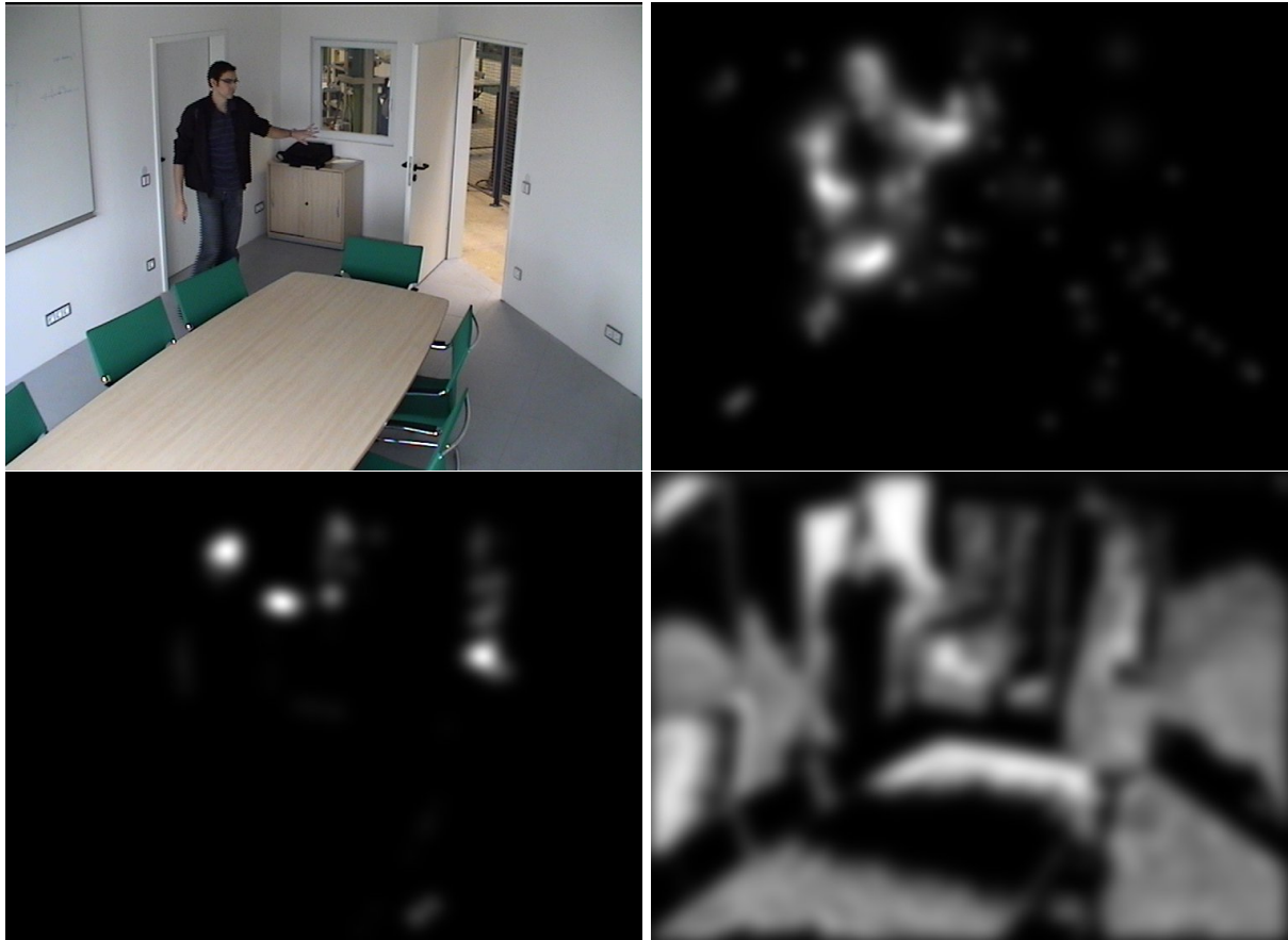
Figure 4: Examples for saliency maps. From left to right, top to bottom: Original image, SIFT saliency, skin saliency (L*a*b* classifier), skin saliency (nRG classifier)
