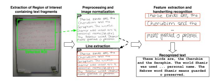
Figure 2. Camera-based whiteboard reading – system overview
