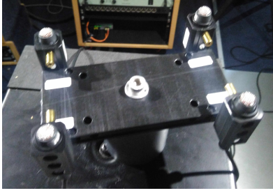
Fig. 3. Smartphone mockup comprised of four microphone mounts attachable to a plastic body.
