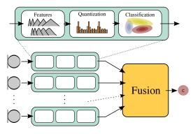
Figure 1: Overview of the proposed method. A three-step BoF approach for acoustic event detection is applied to every source in a sensor network comprised of many microphones, before the results are combined by a fourth fusion step.
