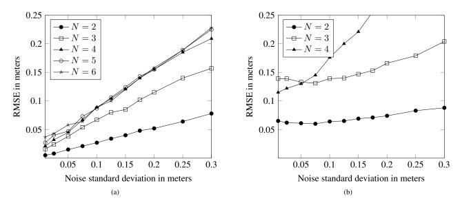
**Fig. 3**: Simulation results for an increasing number of sensors and increasing amount of noise. The results of the proposed approach (a) are shown in direct comparison to the results of the same optimization procedure not using the prior knowledge (b).
