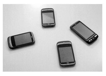
**Fig. 1**: An exemplary ad hoc array comprised of four commercial off-the-shelf smartphones.
