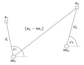
Fig. 2: Array setup depicting the given global orientations  $\varphi_*$ , distances  $d_*$  and the Euclidean distance of the loudspeaker  $s_k$  to the microphone  $m_i$ .
