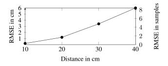
Fig. 5: RMSE for increasing distance of two phones in meters (left axis) and corresponding samples (right axis) according to Eq. (13) for a sampling rate of  $f_s = 48$  kHz.
