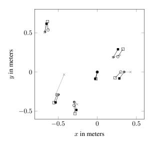
Fig. 4: Exemplary self-localization result for N = 6 smartphones and a measurement noise with standard deviation  $\sigma = 0.1$  m converged after 10 iterations.
