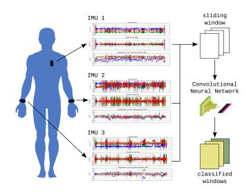
Figure 1. Overview of the proposed approach using an example of three IMUs worn by a worker at both wrists and the torso.
