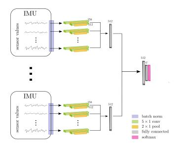
Figure 2. Overview of the proposed IMU-CNN architecture. First, the data of each IMU is processed independently and then the information is joined in a fully connected layer. In the last layer of size c (= number of classes), a softmax classification is performed (*best viewed in color*).
