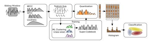
Fig. 1. Overview of the method: Given a window containing an acoustic signal, MFCCs, GFCCs and a loudness feature are computed. The resulting feature vector is augmented by a quantized time coordinate with respect to the window. A GMM is applied for clustering the features of each class in order to learn a supervised codebook. Finally, all features are quantized and the resulting histogram is classified by a multinomial maximum likelihood classifier.
